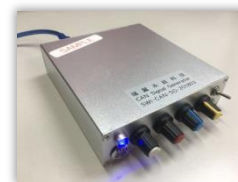
CAN Signal Generator
